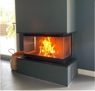
Steel insert with 3 seripgraphics glasses. Small depth of the appliance. Lift up door for wood loading. Interior made in anthracite refractory bricks. Direct connection to outside air. Glass protect system (to keep the glass clean, longer).
